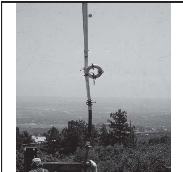
Figure 2: Loop in pump boom
